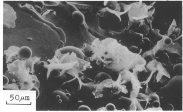
Figure 2 Appearance of flower-like graphite (SEM).
